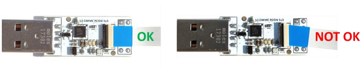
Fig 3. correct insertion of the FFC cable
