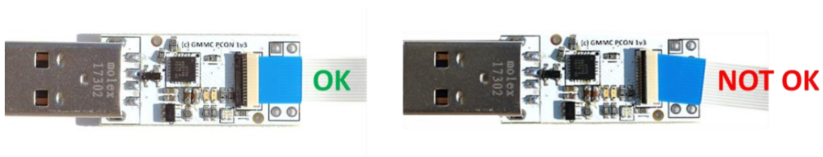
Fig 3 correct insertion of the FFC cable
