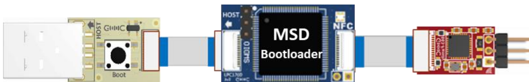
Fig 11 LPC1769 hardware configuration with flashed USB Mass Storage boot loader
