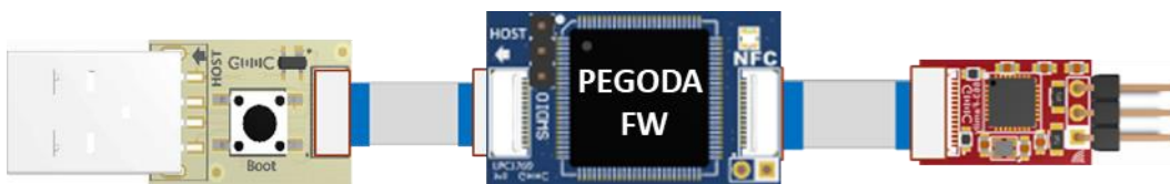
Fig 15 LPC1769 hardware configuration for PEGODA / RFIDDiscover operation
