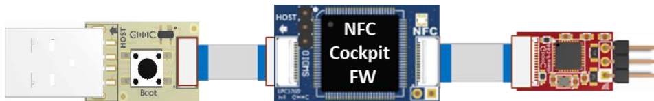
Fig 19 LPC1769 hardware configuration for NFC cockpit execution
