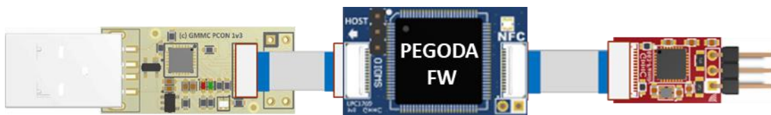
Fig 14 LPC1769 hardware configuration for PEGODA firmware download
