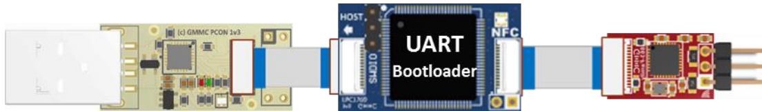
Fig 10 LPC1769 hardware configuration and standard UART bootloader
