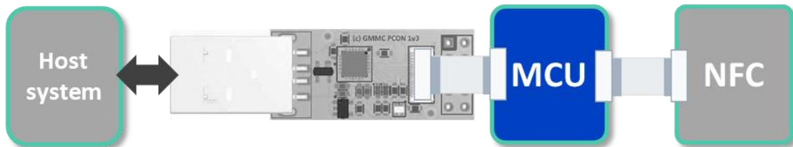
Fig 6. Hardware setup with MCU
