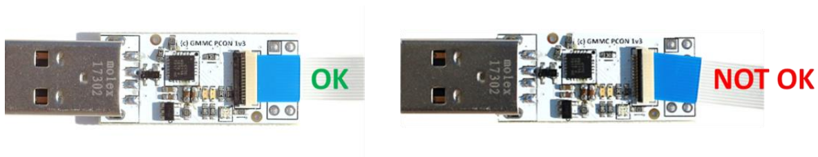
Fig 3 correct insertion of the FFC cable
