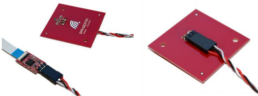
Fig 10. NFC Module – NFC Antenna connection
