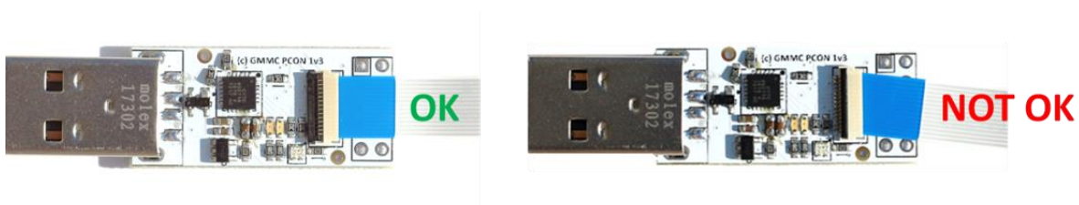
Fig 3. correct insertion of the FFC cable
